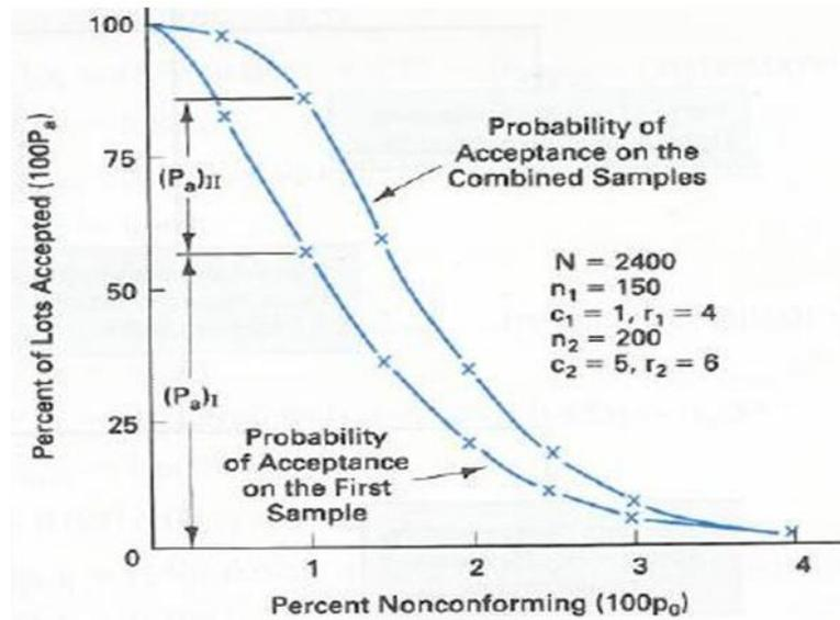
Figure: OC Curve for Double Sampling Plan
