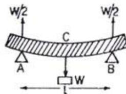
Consider a light beam supported symmetrically on two knife edges A and B at a distance ' $l'$ ' apart with a load W at the middle point 'C' of the beam. The reaction at each knife edge is equal to  $\frac{W}{2}$  in the upward direction.
