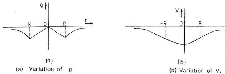
**Fig. 5.7** Graphical representations of variation of field intensity and potential of a solid sphere
