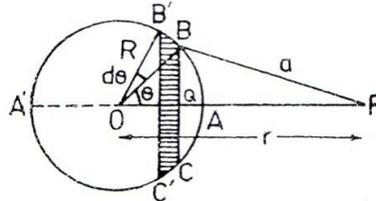
**Fig.5.3.** Potential due to a spherical shell
