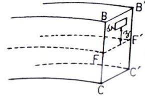
Let a beam ABCD having rectangular cross section be bent in the form of an arc of a circle of radius  $R$  with the centre at  $O$ . Consider a small portion  $ab$  of neutral axis of the beam subtending an angle  $\theta$  at the centre  $O$ .  $a'b'$  is another small portion of a filament at a distance ' $z$ ' above the neutral filament  $ab$ . Before bending  $a'b' = ab$ . After bending,  $a'b' > ab$  since  $a'b'$  is above the neutral surface.
