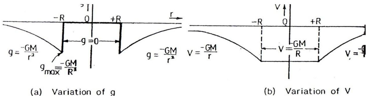
**Fig. 5.4.** Graphical representations of the variation of the field intensity and the potential of a spherical shell
