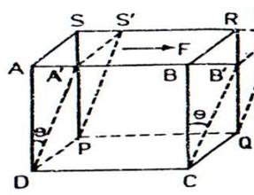
Fig. 3.2 Application of shearing force on a solid cube
