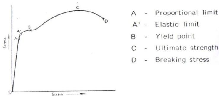
Fig 1.1 The Stress – strain curve for low carbon steelwire
