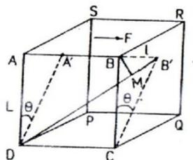
Fig 1.4 Application of a Shearing force on a cube.
