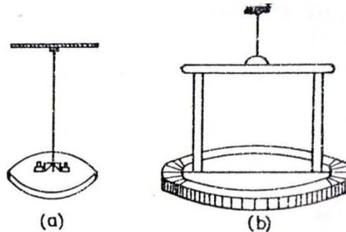
The torsion pendulum is formed by the given circular disc suspended whose rigidity modulus is to be determined. The experiment consists of three parts:
