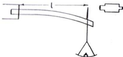
A given rod (or bar) whose Young's modulus is required is clamped firmly and horizontally at one end. A weight hanger is suspended from the free end of it as shown in the above figure. A vertical pin is also fixed firmly to the free end of the rod using wax. A travelling microscope is focussed on the pin and the image of the tip of the pin is made to coincide with the point of intersection of the cross wires.
