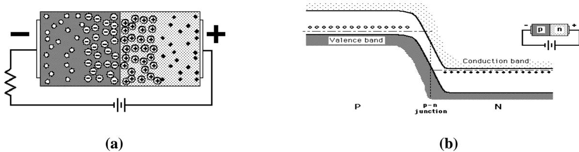
**Fig.2.8 Biasing the PN Junction. (a) Reverse bias (b) Energy band diagram**
